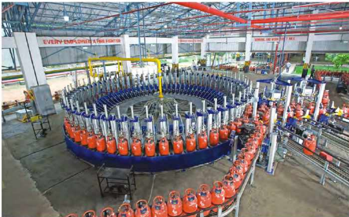
HPCL Flex Speed carousel at Cherlapally LPG Plant HPCL
